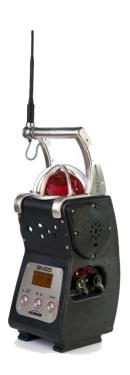
The BM25 packs the benefits of a fixed system area monitor into a rugged, user friendly and transportable instrument.
