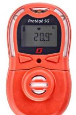
The Protégé SG is a reusable single gas monitor that can be configured to detect 12 gases which provides maximum flexibility to deal with unknown gas hazards. With interchangeable smart sensors the Protégé SG offers maximum versatility in a re-usable solution.
